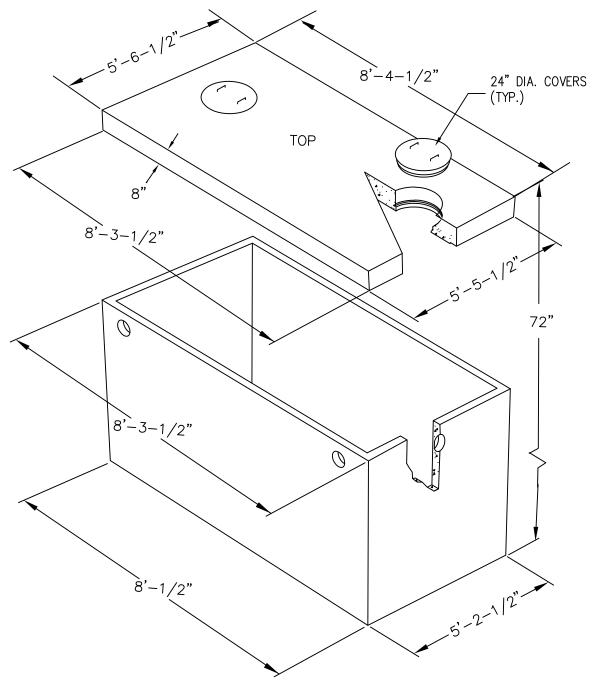
1000 GAL. H-20 MONOLITHIC PUMP CHAMBER
