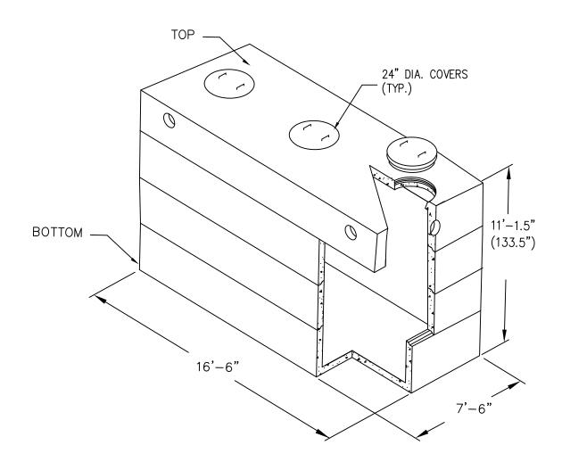
7,000 GALLON PRECAST SEPTIC TANK/H20 AVAILABLE IN 2 or 3 COMPARTMENT
