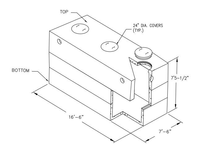
4,000 GALLON PRECAST SEPTIC TANK H20 T4000H AVAILABLE IN 2 OR 3 COMPARTMENT
